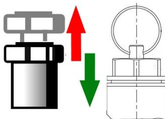
Step 1: Pull the lifting knob / pull-ring upwards until blow-off of the operating medium is clearly audible.
